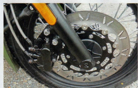
18" wheels. Linked triple disc brakes: front 320mm floating disc, three-piston caliper, sidecar and rear 256mm disc with single piston caliper
